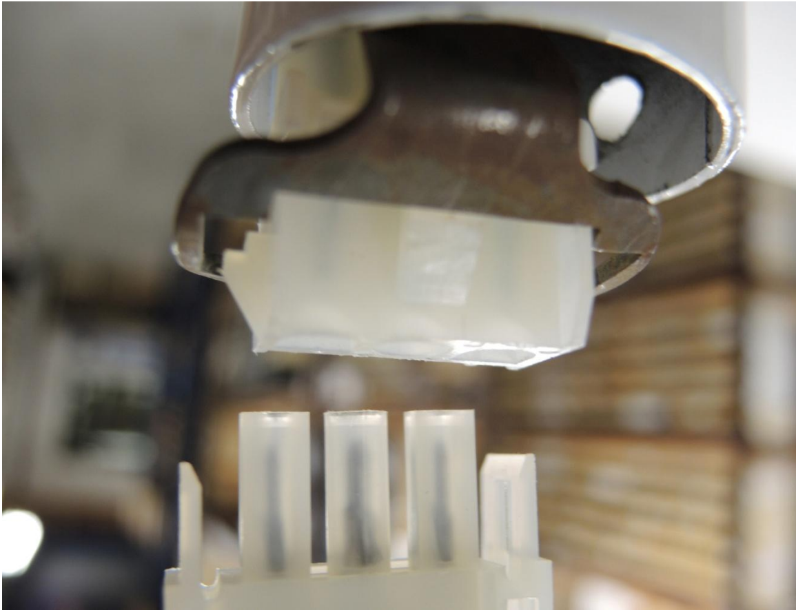
This photo shows the female receptacle (top) of the power cord within the piping and the male plug (bottom) of the power cord for the LED lighting fixture.
